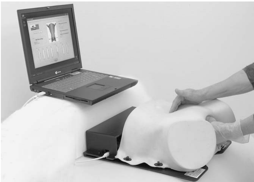
Figure 3 Pelvic simulator, for gynaecological exams, exterior. © The New Visualization and Simulator Technologies Group, Linköping University.
